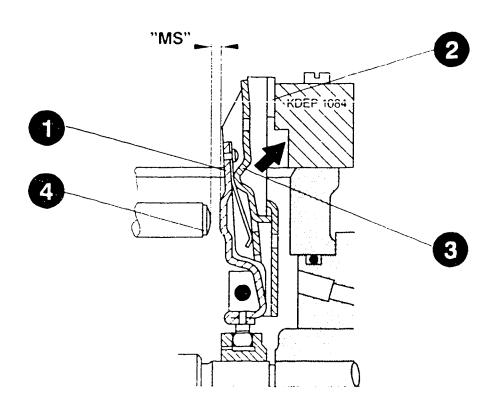
Loosen slotted hexagon nut at governor shaft and turn out governor shaft. Pull out governor shaft until end of thread coincides with outer edge of pump flange (arrow).
